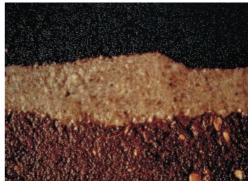
When in contact with water, or just simply in contact with the ground humidity, the natural sodium bentonite turns into a waterproof gel through hydration and expands up to 16 times its initial dry volume while remaining in its waterproof gel state.
